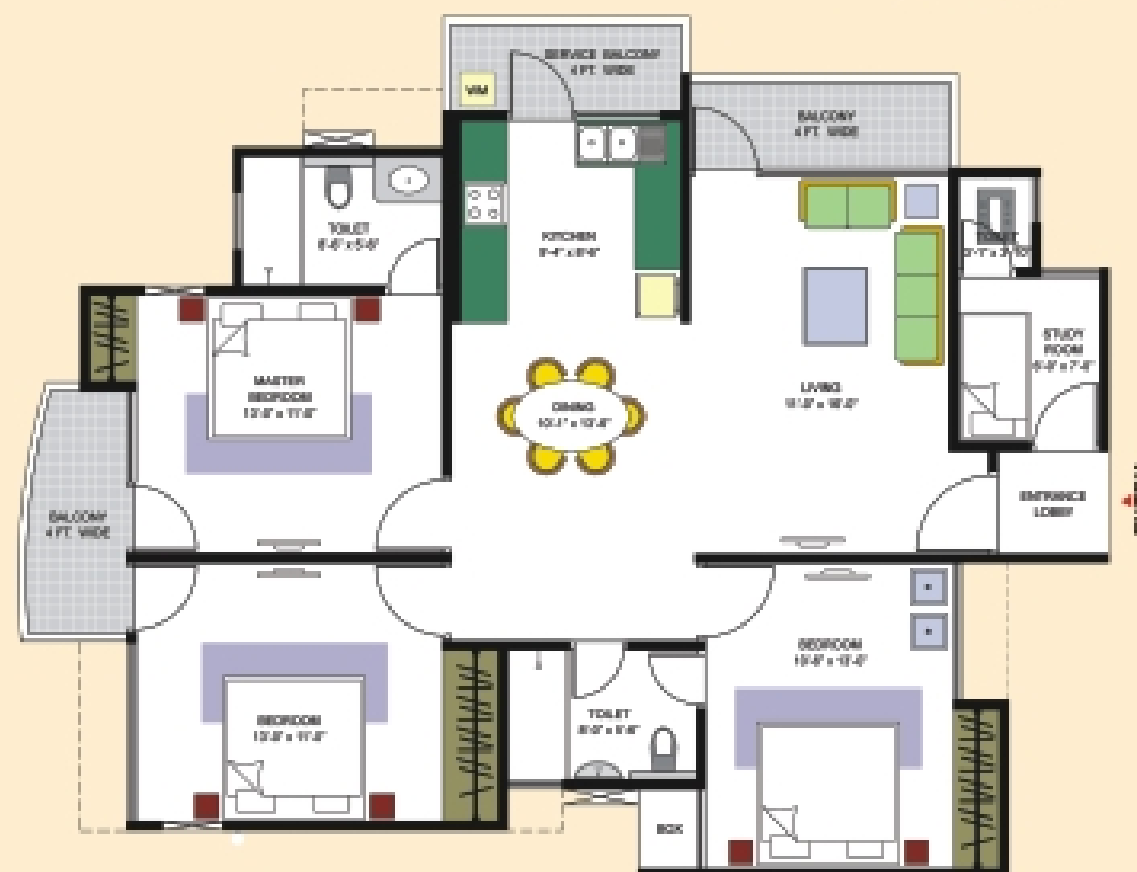
3 Bedroom Apartment + Study / Super Area = 1675 sq.ft. • Living Room • Dining Room • Kitchen with Service Balcony • 3 Bedroom with Sufficient Cupboard Storage • Study Room with Attached Toilet • 2 Spacious Toilet with Accessible Shafts • 3 Spacious Balconies
